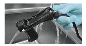
Dry completely with a lint-free cloth. Visibly inspect the entire handpiece for any remaining contamination and repeat the cleaning procedure if needed.
