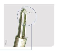
Slivers of the working channel scraped off during clip passage
